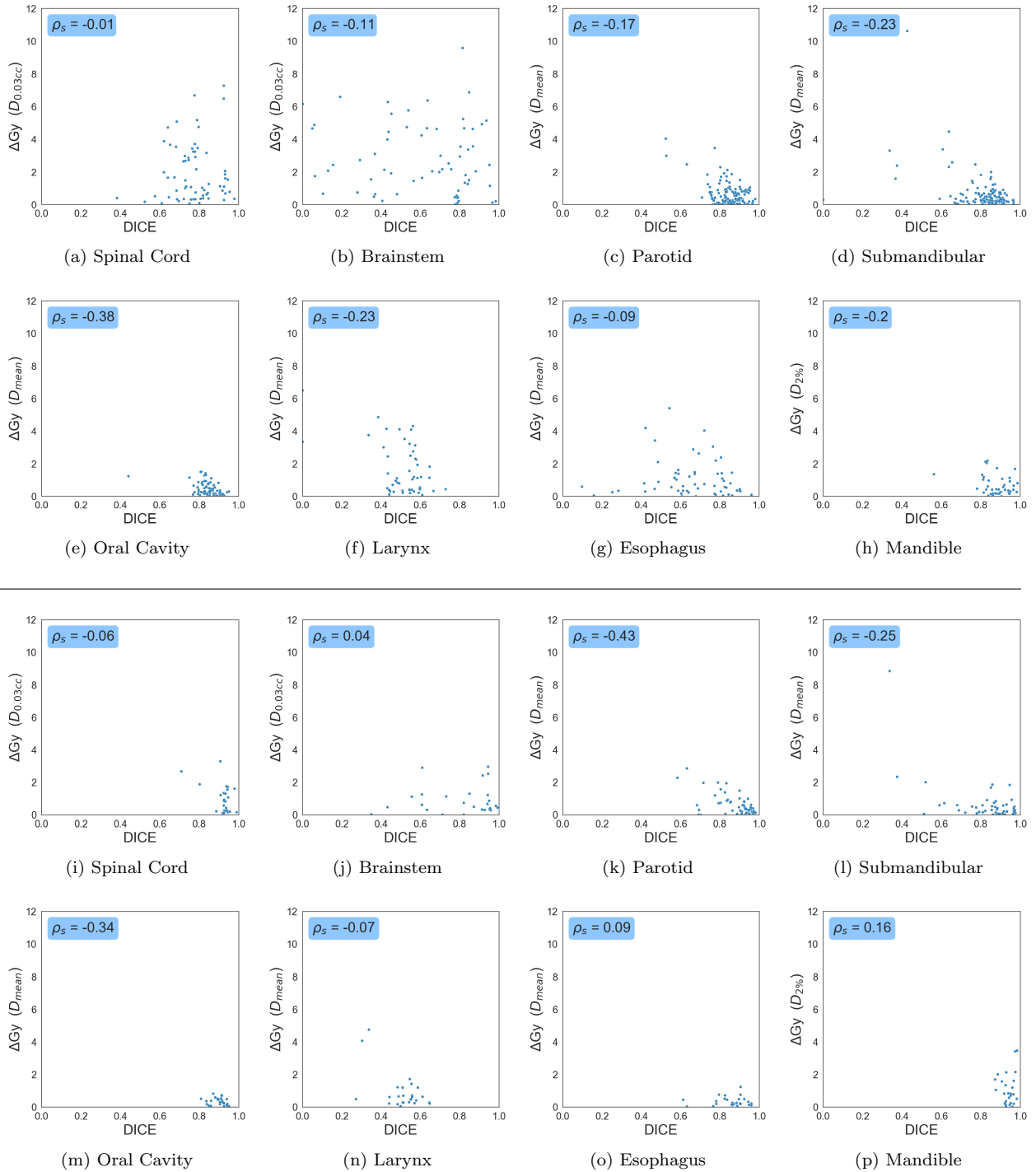
Figure 5: Scatter plots for eight organs-at-risk from the auto-contouring module. Here we plot the DICE (x-axis) against each organs absolute dose metric differences, i.e., |P_{MC} - P_{AC}| (y-axis) for photon (a-h) and proton (i-p) radiotherapy.
