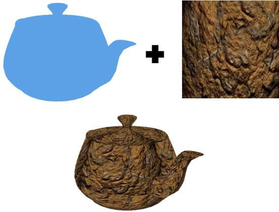
Figure 9. Applying texture to a model within the fragment shader.
