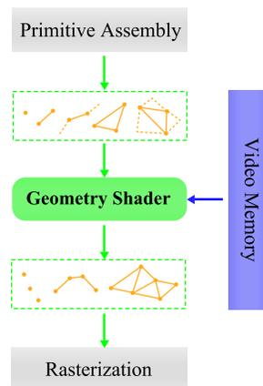
Figure 5. Pipeline Geometry Shader.
