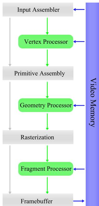
Figure 3. The data flow inside the graphics pipeline.
