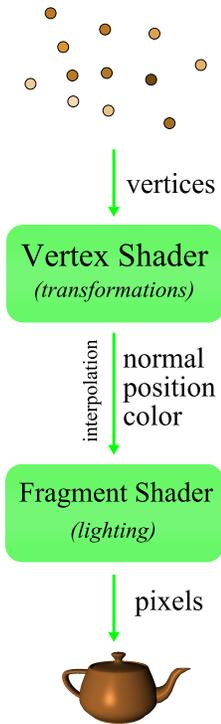
Figure 11. The data flux of the Phong shaders. Note how the lighting operation was postponed from the vertex shader to the fragment shader.
