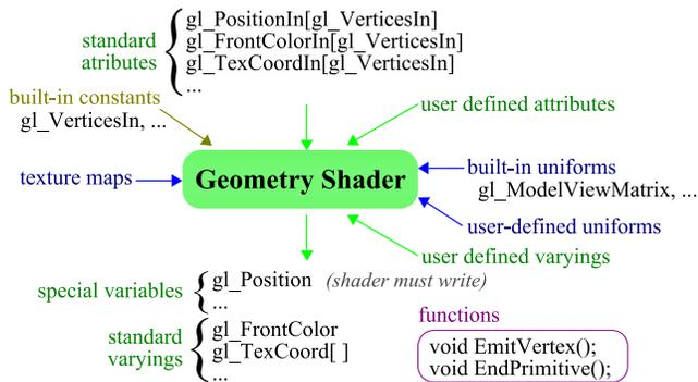
Figure 17. Input/Output summary of the geometry shader.
