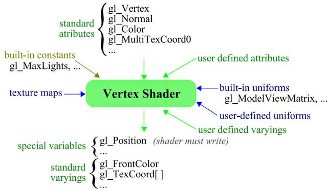
Figure 16. Input/Output summary of the vertex shader.
