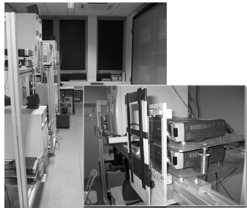
Figure 1: The frame, projectors and driving PCs at the ICWall site.
