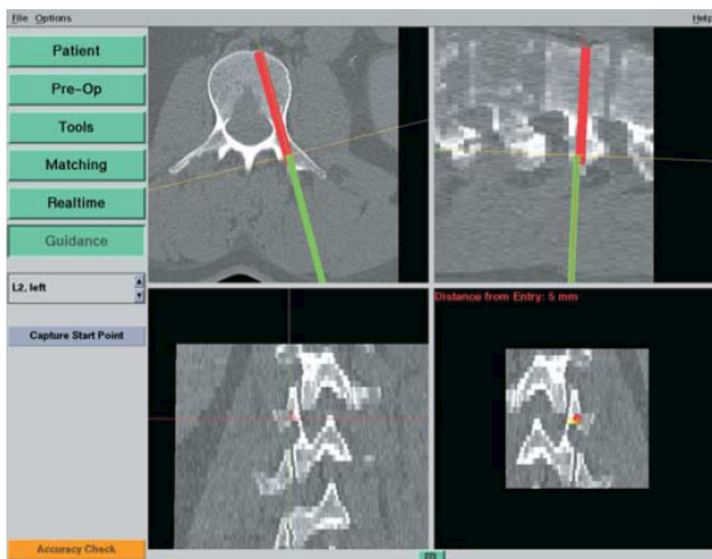
Figure 2.33: CT-based navigation of pedicle screw placement in vertebra L2. The preoperatively planned screw insertion is shown in red and the intraoperatively tracked screw placement instrument is shown in green (Langlotz and Nolte, 2004)
