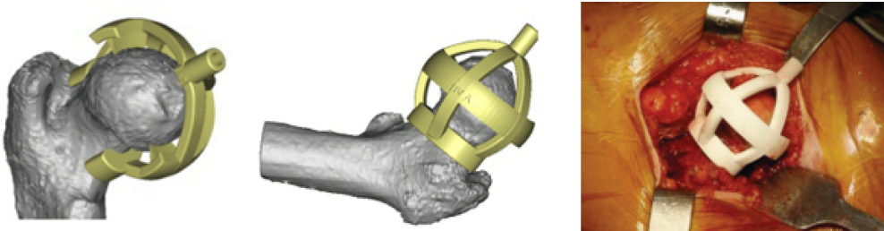
Figure 2.20: Drill guide for hip resurfacing surgery (Raaijmaakers et al., 2010)
