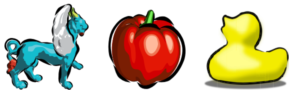
Figure 10: (Left) The “feline” is rendered with regions defined by the visual contour, a shadow boundary and one Lambertian isophote contour. (Center) The pepper model is complex but the contours are simple. It uses two specular and diffuse contours for the pepper itself and one for the stem, respectively. (Right) The duck demonstrates advanced region shading by using blurred fills for its interior regions and shadow.
