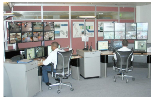
Figure 2: Surveillance control room with a traditional video matrix display arrangement. Operators select sets of individual videos from 2D maps.
