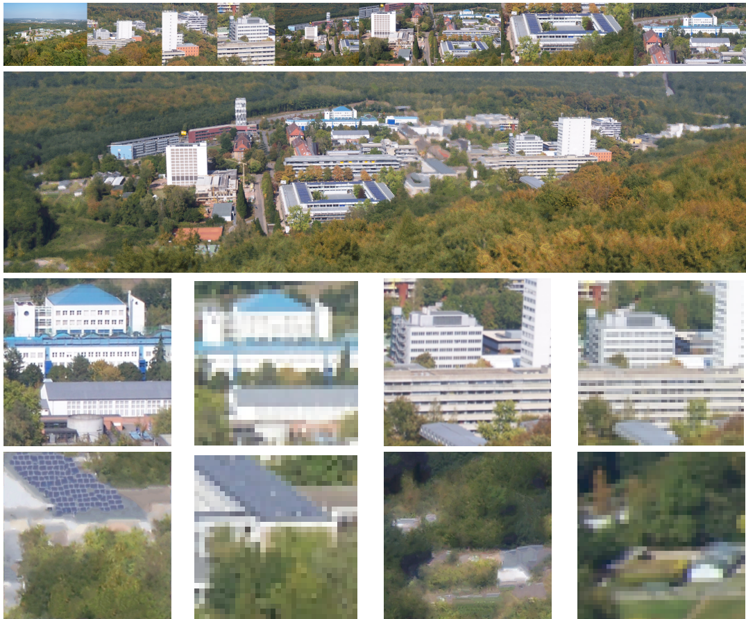
Figure 8: Multiscale-Panorama Stitching: Using 9 input images at various zoom levels, partly overlapping and of varying sizes between 483 \times 525 and 1086 \times 585 our algorithm automatically establishes the dependency graph, scale relations, and blending masks to create a high-resolution panorama image. We upsampled the original panorama with a 683 \times 512 resolution 5464 \times 4096 . 1 st row: Thumbnails of used input images. 2 nd row: Panorama generated by our algorithm. 3 rd row: Two examples of regions incorporating information from the detail images and the respective part in the original panorama image. Notice that the given details have been faithfully included in the high resolution panorama. 4 th row: Two examples for enhanced details next to their respective parts from the original panorama image. Both examples show regions where no direct correspondence relation with respect to the input images existed. Our solution adds subresolution detail, invisible in the original input image (here, with 64 times more pixels). In many cases, plausible details are added by our algorithm, e.g., the solar panels on the roof (left). The texture synthesis step is especially useful for small scale and repetitive structures like the leaves of the trees. Nonetheless, if no sufficient detail information is available from other parts of the input images, it is not possible to reconstruct semantically meaningful structures like the houses on the right faithfully.
