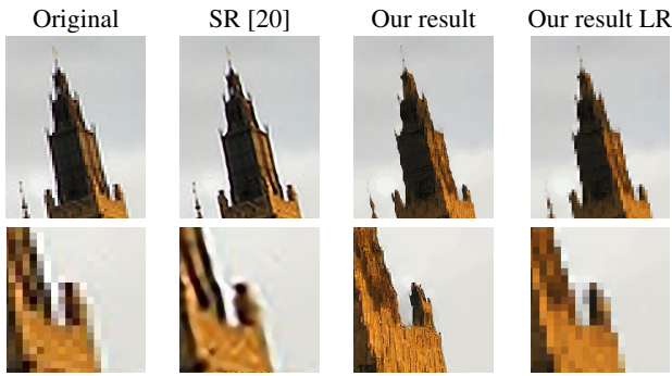
Figure 11: Comparison to Super-Resolution in the Big Ben scene. Super-Resolution approaches upsample images by guaranteeing equivalence to the original image after downsampling. Our approach instead assures similarity to the original, this loosened constraint allows the algorithm to add new plausible details to the image. From left to right: Original image, upsampled image by three octaves using the method described in [20], upsampled image using our proposed algorithm, downsampled result of our algorithm. None of the input images contained a close-up view of the turret.
