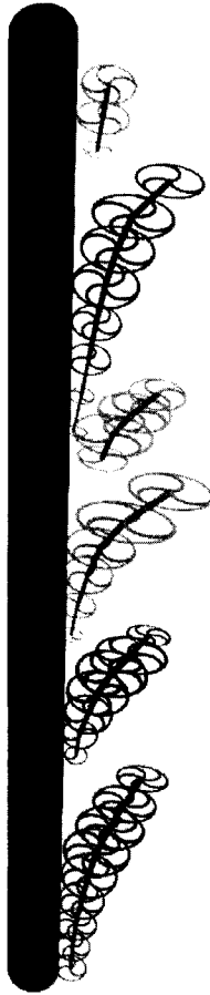
Figure 8.28: The 3D vortex graph obtained by tracking 2D vortices in space, figure is shown in color on the backside of the cover.
