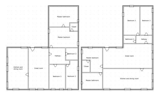
Figure 5: Two examples of a more complex floor plan, built up of a public zone with a great room and kitchen and dining room, a private zone with a master bedroom and walk-in closet, master bathroom and a private zone with a hallway, a bathroom and two bedrooms.
