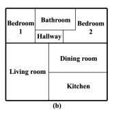
Figure 2: This is an example of a hierarchic subdivision of a building. (a) shows a building subdivided into two areas, (b) shows these areas subdivided into their required rooms.
