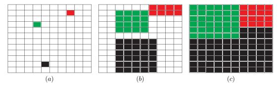
Figure 3: Example for the room expansion algorithm: (a) initial room positions (b) rectangular growth (where rooms reached their maximum size) (c) L-Shape growth.
