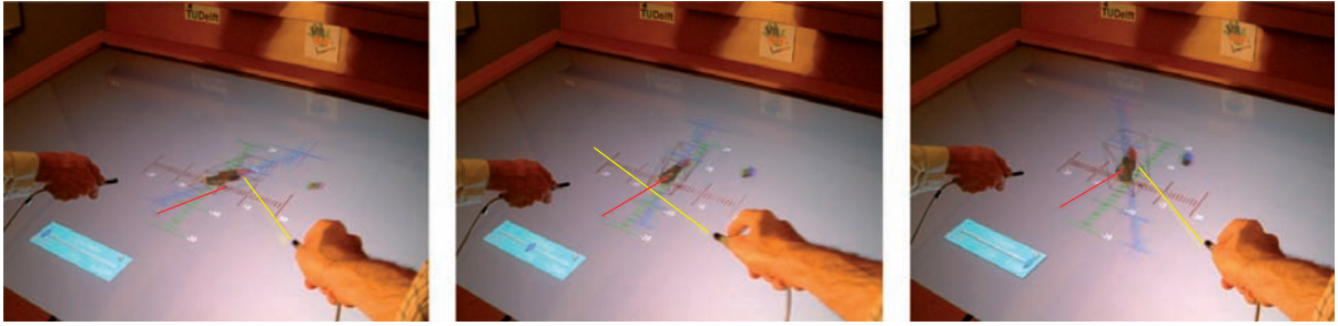
Figure 1: Demonstration of our method in a two-user scenario at the Virtual Workbench. The scene is rendered from the viewpoint of the left user (left image), the right user (right image) or a dynamic, average viewpoint (middle image). Although objects may not appear in the correct perspective for either user in the averaged viewpoint, interaction with the distorted environment is still possible, as each user has personal, corrected interaction tools.
