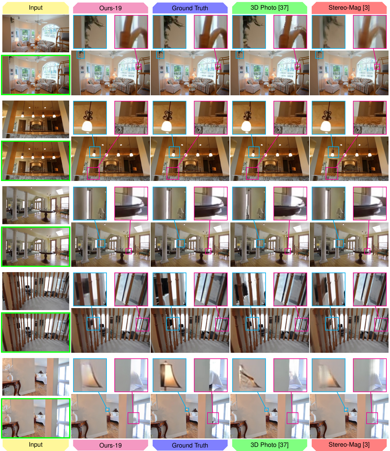
Fig. 20: Extrapolation comparison of our method with 19 planes (Ours-19) against ground truth, 3D Photo [37], and Stereo-Mag [3]. The input frame closer to the target frame is marked in green for easier comparison.
