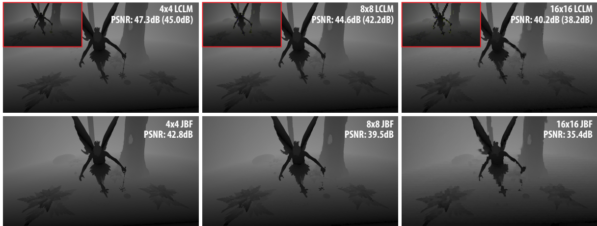
Figure 7: Quality for various upsampling levels. Downsampled depth images are in red insets. Our (LCLM-top) vs. a joint-bilateral method (JBF-bottom) on uncompressed sparse depth. PSNR numbers in parenthesis refer to our method without \hat{d}^c (not shown). Our quality is consistently higher. For 4 \times 4 upsampling, both perform well, but JBF loses some fine geometry.
