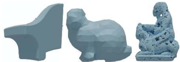
Figure 28: Limit cases (l.t.r.): Sharp edges on artificial object, under-sampled regions (bunny ears) not reconstructed (down-sampled to 1%), and extreme outlier levels (40%).
