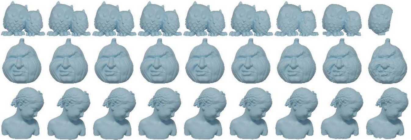
Figure 11: Result of our algorithm on down-sampling. L.t.r.: 100%, 80%, 60%, 40%, 20%, 10%, 5%, 1%, 0.05% of points are retained using ReMesh simplification. Models taken from [HWW*22] (originally from Thingi10k [ZJ16]) and aim@shape.
