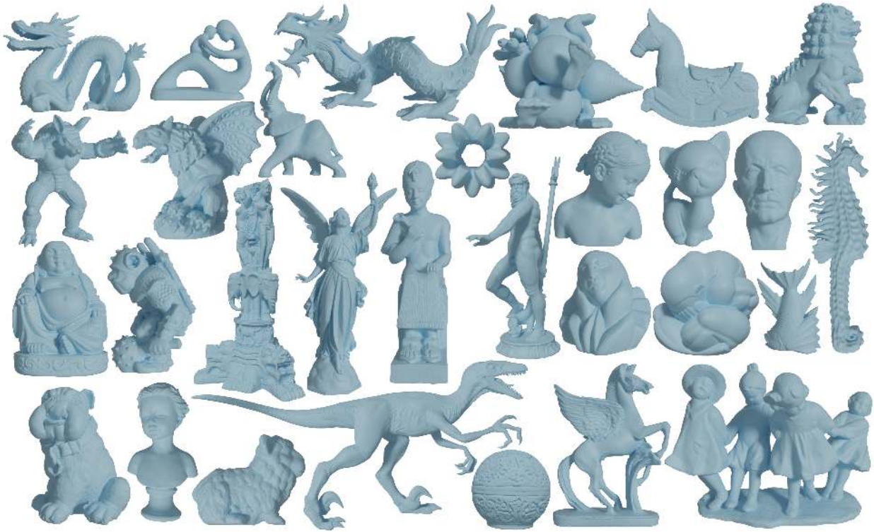
Figure 20: Automatically-generated Watertight triangulations via GLOBAL BALLMERGE for point clouds (up to 3609k points) from aim@shape and Stanford ([TL94],[CL96]) with challenging features (e.g., corners, ridges, and close surface sheets).
