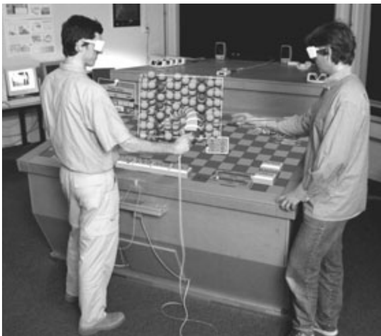
Figure 4.47: Particle steering of \beta -Alumina electrolyte with the spring manipulator on the Workbench (see also the Color Section)
