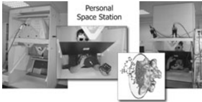
Figure 2.12: The user can manipulate the protein model with his left hand, holding a cube with markers. The protein geometry can be clipped by using a clipping tool in the right hand. [Image source: CWI (Netherlands)]
