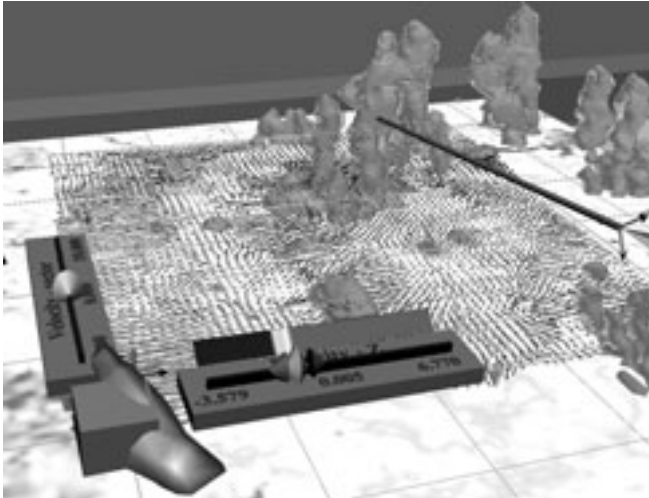
Figure 5.18: Atmospheric visualization: the direct vector slicer shows the flow momentum around the cumulus clouds (iso-surfaces of liquid water concentration).
