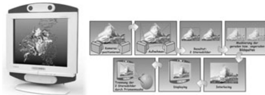
Figure 2.6: Autostereoscopic display with optical camera-based eyeball tracking [Image source: Dresden3D]
