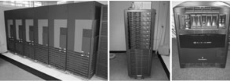
Figure 6.16: Supercomputers at HP \alpha C. From left to right: Cray T3E, Beowulf Linux cluster and SGI Origin 2000
