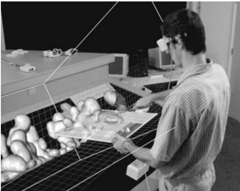
Figure 6.54: The user performs a two-handed exploration of the cloud data. The non-dominant hand holds the Plexipad with clipping planes and direct data slicer, while the dominant hand navigates and probes the data (see also the Color Section).
