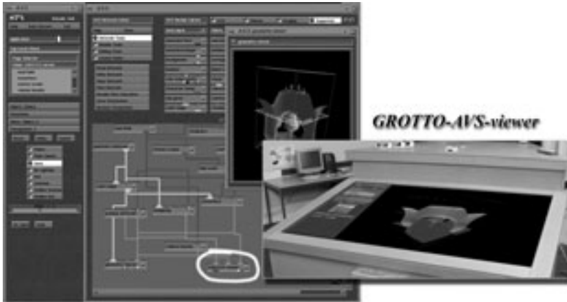
Figure 3.13: Grotto-viewer for AVS 5.0: a visualization network of AVS on the computer screen (left), a view on the Workbench (right)
