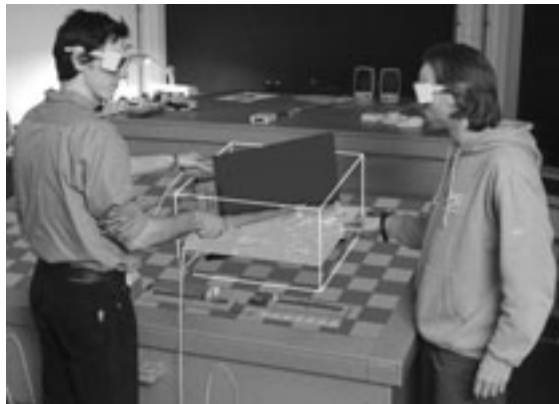
Figure 5.1: Two-handed exploration tools in data visualization on the Virtual Workbench (see also the Color Section)
