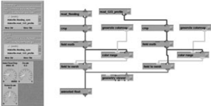
Figure 6.4: Visualization network of the prototype 3D visualization of flooding data in AVS 5.0
