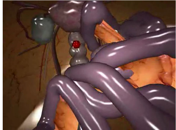
Figure 11: Example application of collision detection (intestinal surgery simulation). The objects in this case are highly deformable. Both self-collisions and collisions between different objects must be detected and handled. (Screenshot courtesy L. Raghupathi, L. Grisoni, F. Faure, D. Marchall, M.-P. Cani, C. Chaillou [RGF*04].)
