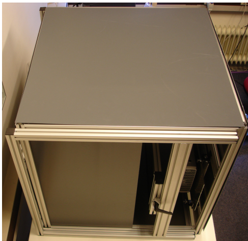
Figure 7: PDRIVE ready for transport. The upper, projector box has been placed within the base frame.
