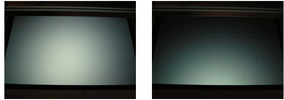
Figure 8: Variation in image brightness between the back projector (left) and the front projector (right) while projecting a uniform, gray image as seen from the user's point of view with factory default settings for the projectors. Hot spots in both images are clearly visible. See Figure 2 for an illustration of the projector placement. The back projector (left) produces a brighter and more uniform image because the image is being projected "towards" the user. The front projector (right) produces a much darker image with a hot spot close to the user because the image is being projected "away" from the user.
