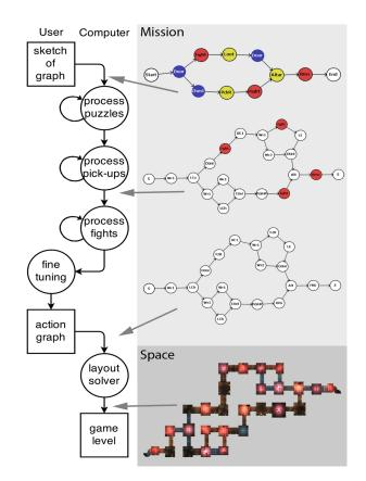
Figure 1: A model of the action graph generation process. Left: The squares represent meaningful products, the circles represent transformation modules. Right: These figures show the data representation during the generation process. The colored nodes in the graphs can be transformed, the white nodes are leaf nodes. The bright rooms in the resulting game level are based on the graph, the dark rooms are fillers created by the layout solver.
