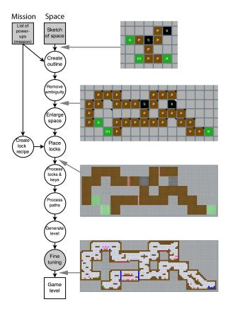
Figure 2: Model of TickTick++ level generation process. Left: The squares represent meaningful products, the circles represent transformation modules. The grey shapes represent the designer's steps. Right: These figures show the data representation during the generation process.
